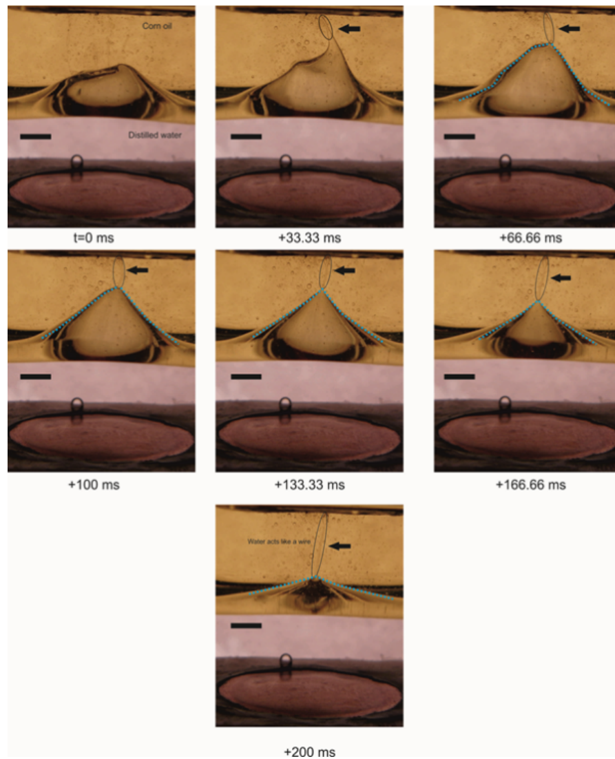
Figure 6. The procedure of discharging distilled water into oppositely charged electrode ( E=219.88 V/mm, scale bar= 5mm)
