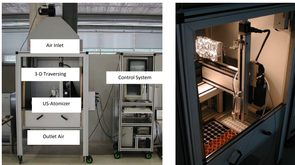
Figure 2: Flow chamber with control system (left) and traversing system above the seedling trays (right)
