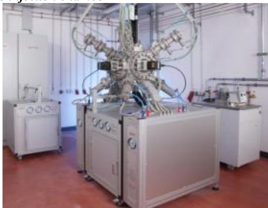
Figure 5. High-pressure and high-temperature injection chamber OptiVeP
