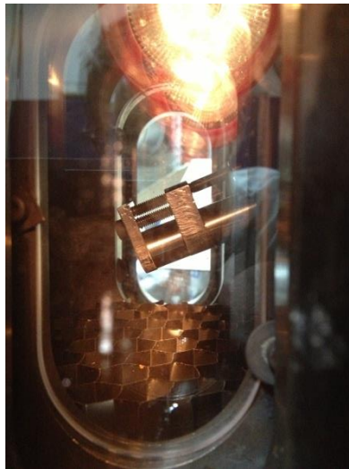
Figure 2: Early prototype of experimental injector mounted in high pressure/high temperature vessel.
