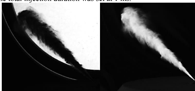
Figure 8. Injection of a GtL-fuel ( p_{inj.} = 80 MPa; T_{inj.} = 323 K; t_{vSOI} = 1000 \mu s) into a low-pressure, low-temperature environment ( p_{chamber} = 1 MPa; T_{chamber} = 473 K)
