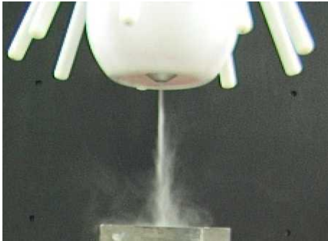
Figure 6: Ultrasonic atomizer with HV needle electrodes
