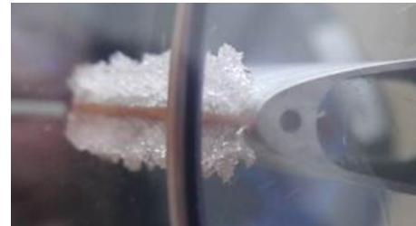
Fig. 8 - Exemplary ice shape generated with the spray bar system on a NACA 0012 aerofoil
