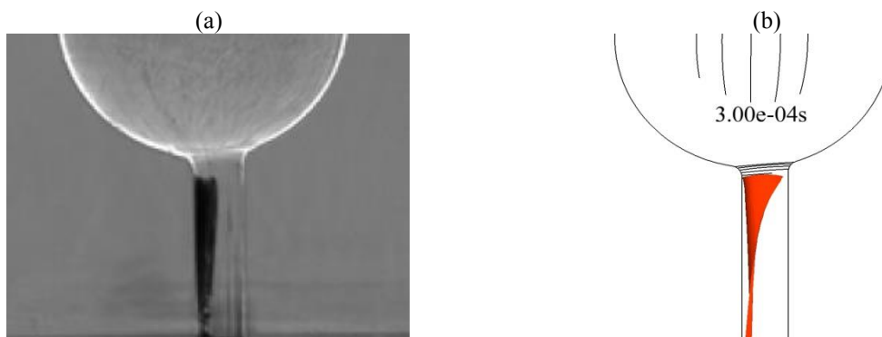
Figure 4 : Qualitative comparison of the numerical and experimental cavitation regions. (a) Shadow-image obtained in the framework of NADIA-BIO project. (b) A volume fraction iso-value equal to 0.5 is used for delimiting cavitation region
