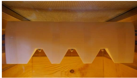
Fig. 6 - Top view of the spray bar system with three nozzles
