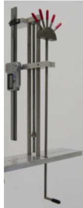
Fig. 13 - Detail view of the traverse unit with a 3D probe
