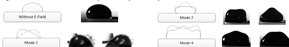
Figure 6: Typical oscillation modes of water droplets under the impact of an alternating electrical field
