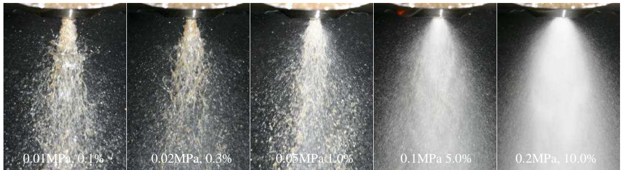
Fig. 4. Spray structure of effervescent atomizer at varying air gauge pressure and GLR.
