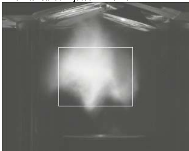
Crank Angle: 139.2° ATDC Time After Start of injection: 1.60 ms 2000 rpm
