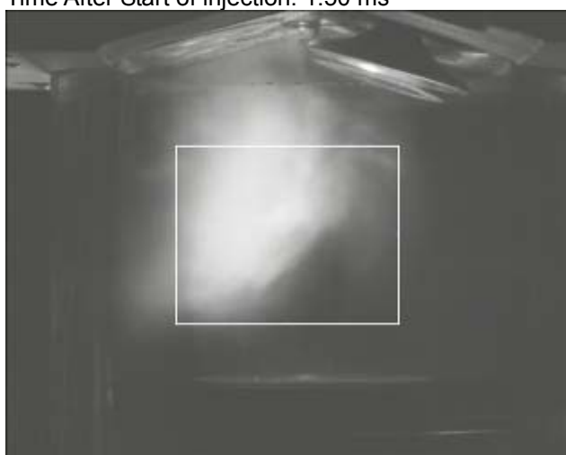
Crank Angle: 120.0° ATDC 3500rpm Time After Start of injection: 1.42 ms
