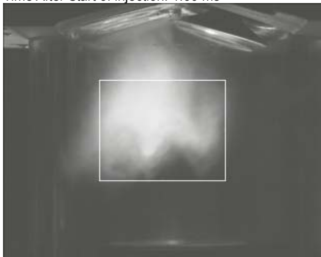
Crank Angle: 152.0° ATDC Time After Start of injection: 1.52 ms 3500 rpm
