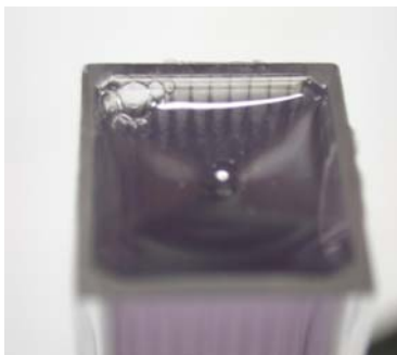
Fig.9 Collagen gel with single phase impingement- gas flow through the central channel
