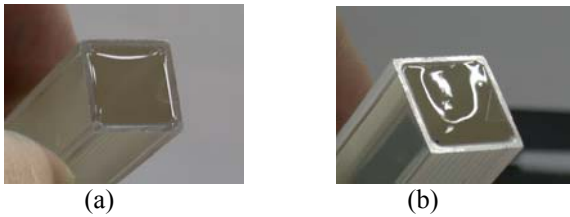
Fig.8 Collagen gel with single phase impingement- gas flow through the side channel (a) Before gas impingement, (b) After gas impingement
